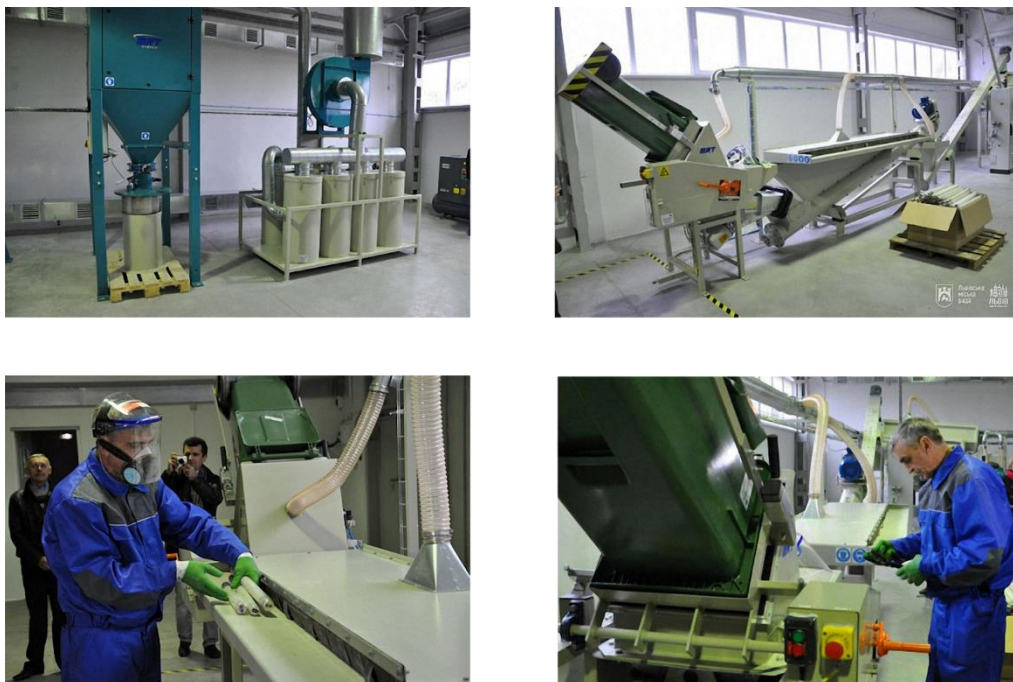
Figure 5.1.2. The decontamination equipment for mercury lamps and other items containing mercury vapor [9]
