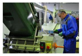
**Figure 7.** The decontamination equipment for mercury lamps and other items containing mercury vapor [7].
